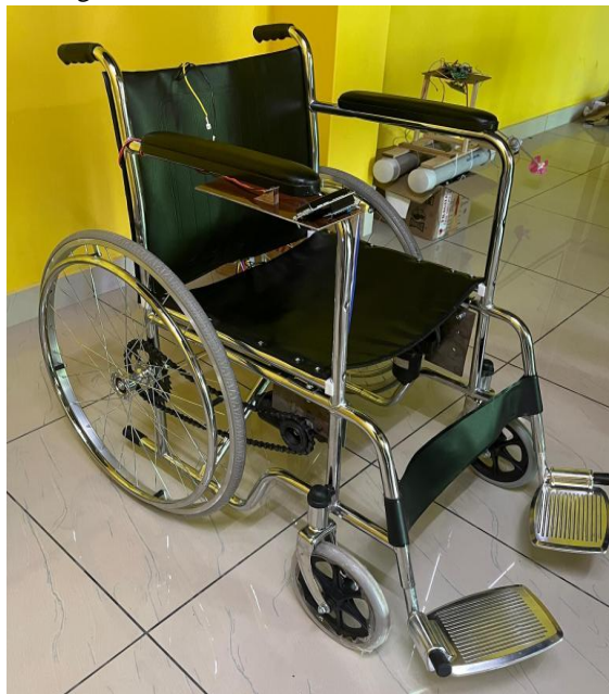
Fig 8 Gesture controlled smart wheel chair
