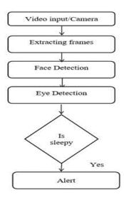
The Driver Drowsiness system is developed using concepts based on invasive machine vision. Here, a webcam that can be used to identify the driver's face is focused on his face. Once the face has been identified,
