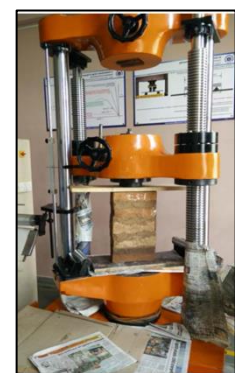
Fig. 5. Test setup of masonry prism
