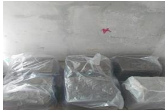
Figure. (3): a) GPC specimen casting b) Curing of specimens under plastic covers
