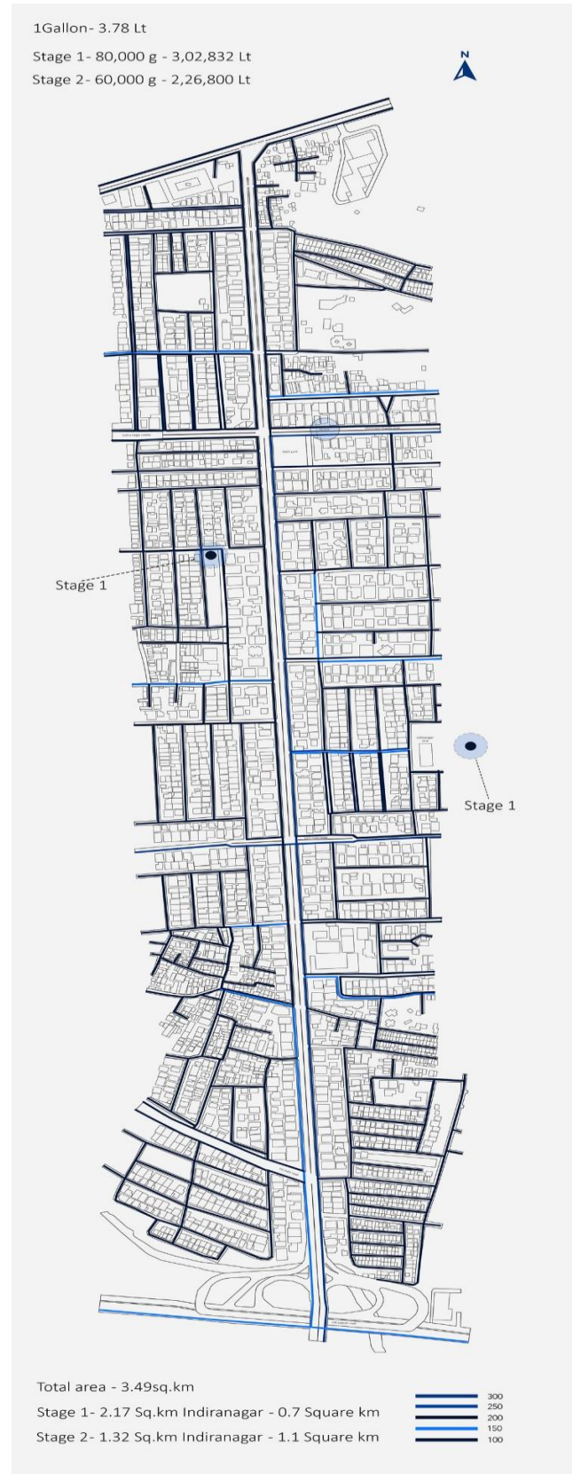
Figure 2. showing water supply network
