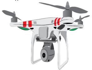
Unlike conventional helicopters, quadcopters do not usually have cyclic pitch control, in which the angle of the blades varies dynamically as they turn around the rotor hub. In the early days of flight, quadcopters (then referred to either as *quadrotors* or simply as *helicopters*) were seen as a possible solution to some of the persistent problems in vertical flight.
