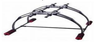
Some of the pilots prefer leg height landing gear in the high grass areas to prevent any mishap while landing. 7. Receiver:
