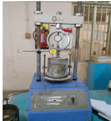
Fig. 2 California Bearing Ratio Test
