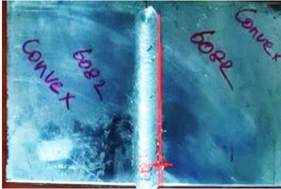
Fig.11 Angle Distortion of Convex Shoulder Tool
