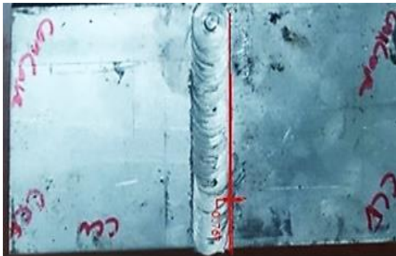
Fig.12 Angle Distortion of Concave Shoulder Tool
