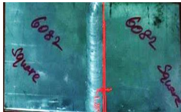
Fig.10 Angle Distortion of Square Shoulder Tool
