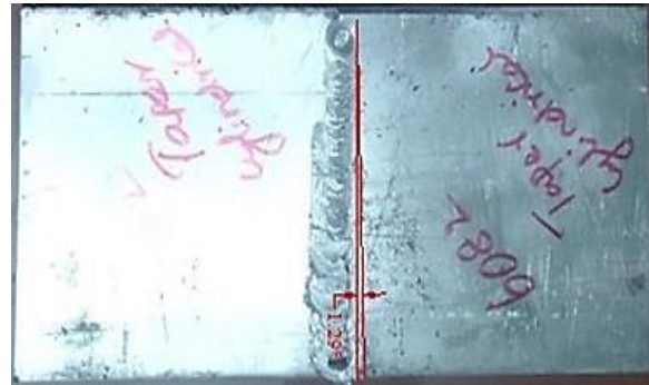
Fig.9 Angle Distortion of Taper Cylindrical Shoulder Tool
