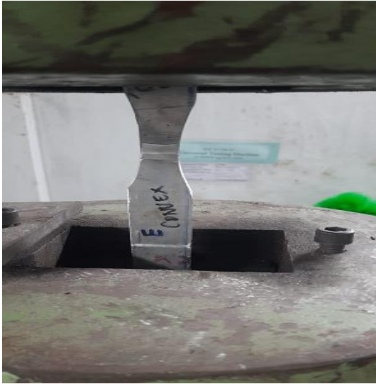
Fig.6 Tensile Test on Specimen
