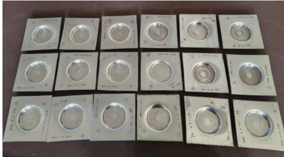
Fig 5: 18 formed GI sheets
