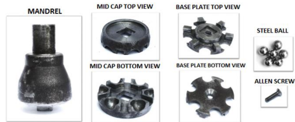
Fig 2: MPIF tool components
