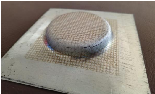
Fig 6: Fracture in formed sheet
