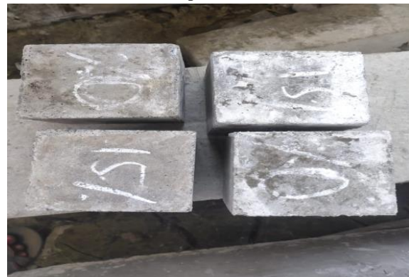
FIG 3 Sulphate attack test
