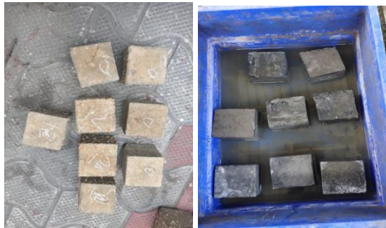
FIG 2 Acid attack test
