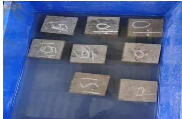
FIG 1 Water absorption test
