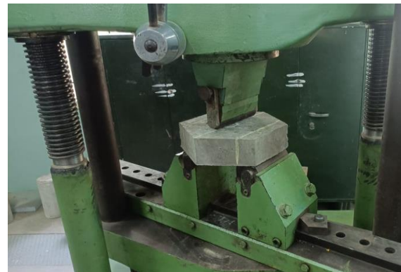
FIG.2 CENTRE POINT LOADING
