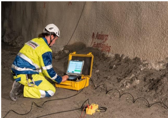
Figure 3-(ii) Simple installation, process for receiver recording & unit with system ( TSP 303 Plus ).
