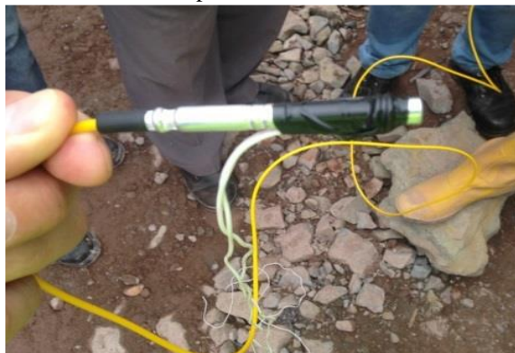
Figure 4 Detonator cap with wrapped round wire (white) that gives the accurate recording trigger in the moment of blast (WBT-mode).
