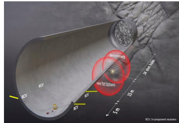
Figure 2. Standard TSP measuring layout with 24 explosive charges are being shot one by one with closed to tunnel drive face on right or left tunnel walls. Four receivers arranged further back pick up arriving waves.
