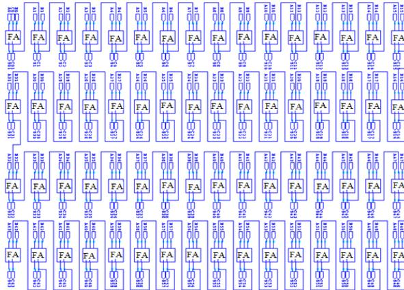
Figure 7:- 64-Bit Ripple Carry Adder
