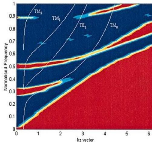
Fig. 10. Dispersion diagram for TM polarization of the PBG configuration under study as a function of  $kz$  together with the dispersion diagram for the surface-wave modes of the
