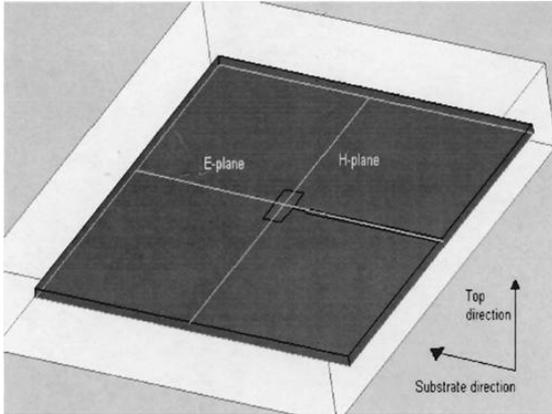
Fig. 4. The conventional patch antenna on a substrate with a dielectric constant of ten.
