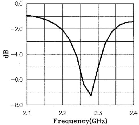
Fig. 12. Input return loss ( ) for the antenna patch on a PBG substrate.
