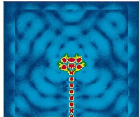
Fig. 7. Surface plot of the electric field of the patch-antenna configuration. Red signifies maximum power while dark blue signifies minimum power.
