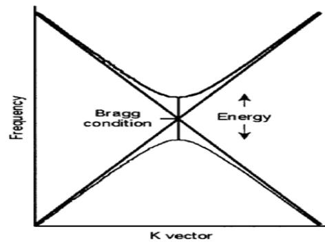
Fig. 1. Plot showing an example of the dispersion relation and the Bragg condition.
