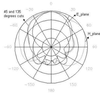
Fig. 13. Far-field radiation pattern from the patch antenna on a PBG substrate. Each division corresponds to 10 dB.
