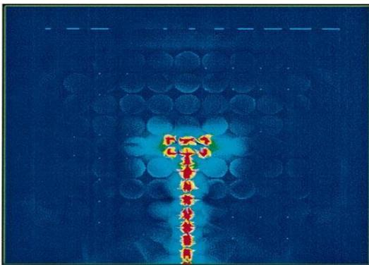
Fig. 14. Surface plot of the electric field in the PBG patch-antenna configuration. Red signifies maximum power while dark blue signifies minimum power.
