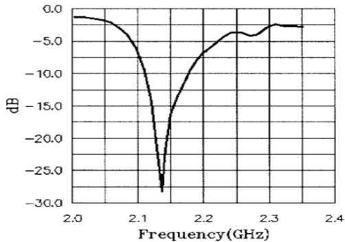
Fig. 5. Return loss ( ) for the conventional patch antenna.
