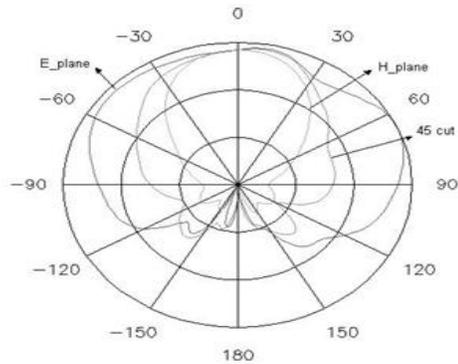
Fig. 16. Far-field radiation pattern at 2.23 GHz from the PBG patch. Each division corresponds to 10 dB. The maximum directivity is 9 dB.
