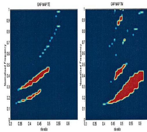
Fig. 9. (a) Gap map for TE and (b) TM polarizations in the case of air columns in a dielectric substrate with "r = 10.
