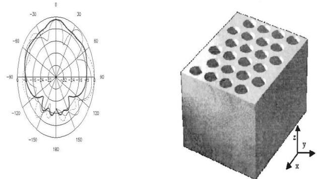
Fig. 6. Far-field radiation pattern from the conventional patch antenna. Each division corresponds to 10 dB. The blue line signifies the H-plane cut and the green line signifies the E-plane. The red and pink lines are the 45 and 135 cuts.
