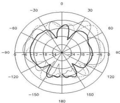
Fig. 15. Far-field radiation pattern at 2.23 GHz from the normal patch. Each division corresponds to 10 dB. The maximum directivity is 8.15 dB. The thick solid line is the H-plane cut, the thin solid line is the E-plane, and the dashed line is the 45 cut.
