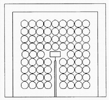
Fig. 11. Patch antenna on a PBG substrate formed by four holes in a square lattice with dielectric constant of ten.
