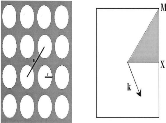
Fig. 3. PC made using a square lattice. (Right-hand side: Brillouin zone of this square lattice). The irreducible zone is depicted in the dark shading.
