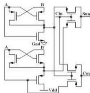
Fig. 3: 10-Transistor full adder circuit
