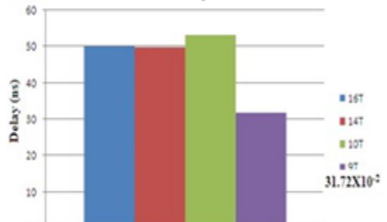
Figure.12. Comparison of Propagation Delay for Carry
