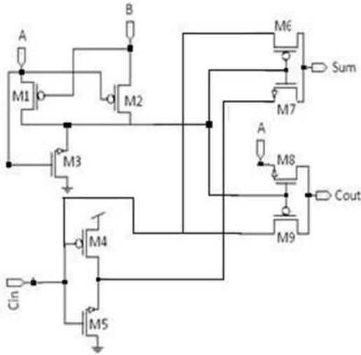
Fig. 4: Proposed full adder circuit
