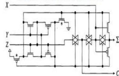
Fig. 2: 14-Transistor full adder circuit
