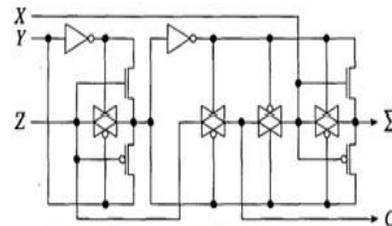
Fig. 1: 16-Transistor full adder circuit
