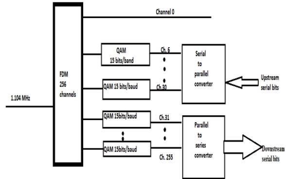
upstream. The channels 31 to 255 are allowed for downstream data transfer and control. Out of 255 channels, one is reserved for control and remaining 224 are reserved for data. The downstream bit rate is  $224 * 4 \text{ KHz} * 15 = 13.4 \text{ Mbps}$ .
