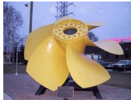
Fig3, A propeller type Runner(21 MW)
