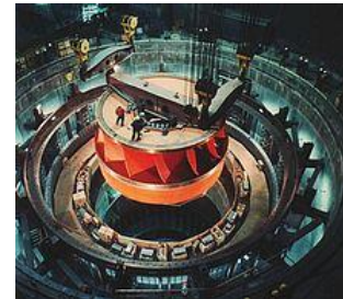
Fig2, Francis turbine Runner (750 MW), installed at Grand Coulee Dam, USA
