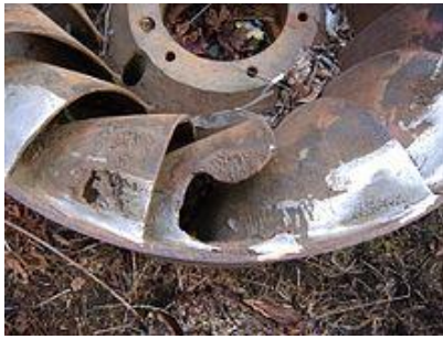
Fig1, Francis turbine, showing pitting corrosion
