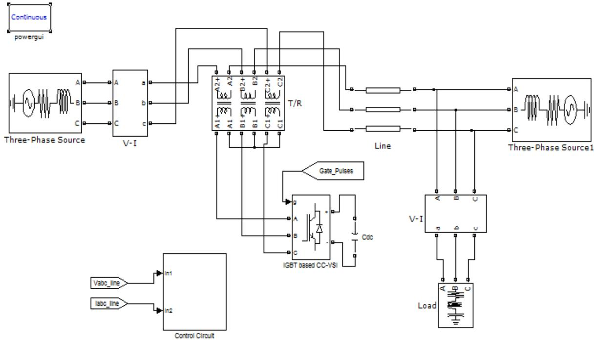
**Fig.2 Schematic System with SSSC**
