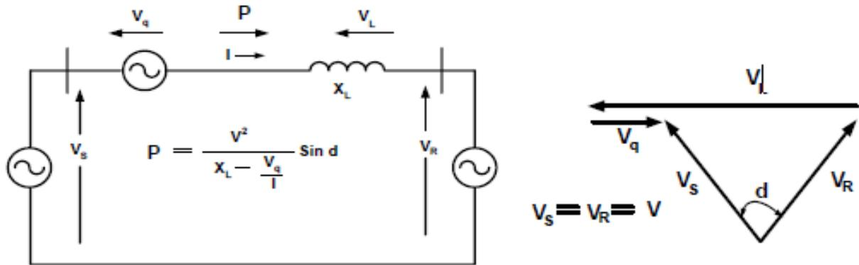
**Fig.1. Elementary two-machine system with an SSSC and the associated phasor diagram**
