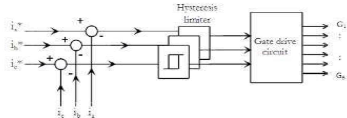
**Fig.4 Schematic of current controlled PWM**
