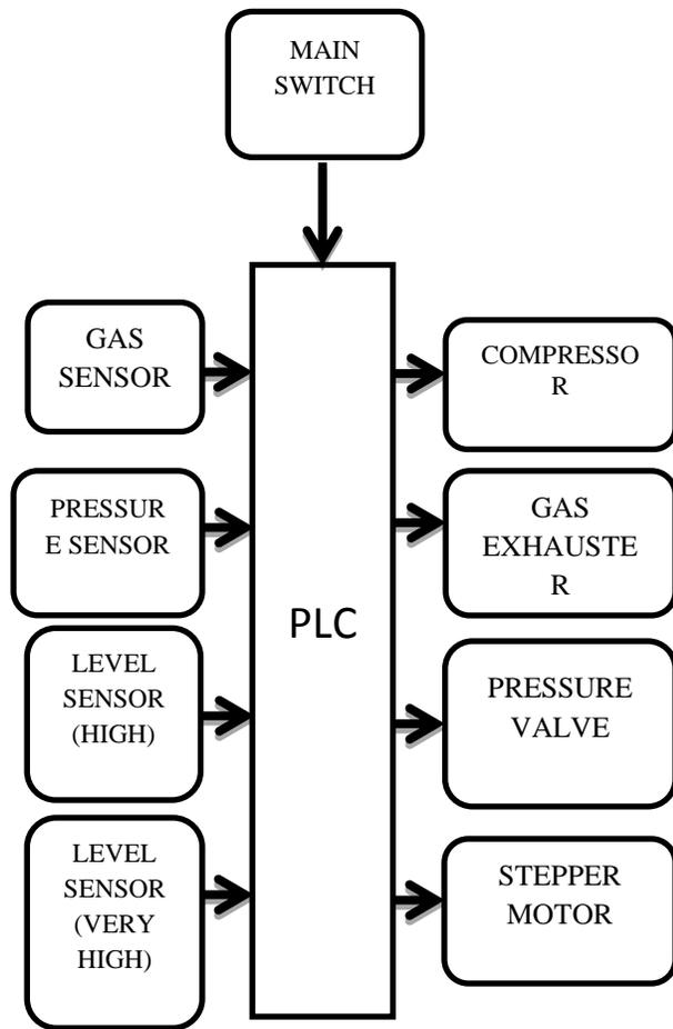
**Fig.1 Block diagram for automatic drainage water pump monitoring and control system using PLC**
