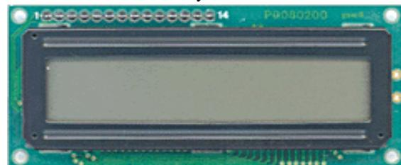
**Figure 10. 16x2 LCD Display**
