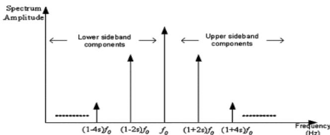
Fig.1. Sideband frequencies around the fundamental line frequency.
