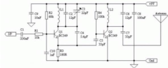
Circuit diagram of low power fm transmitter
