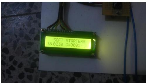
**FIG 3.2 VOLTAGE AND CURRENT MEASUREMENT**
