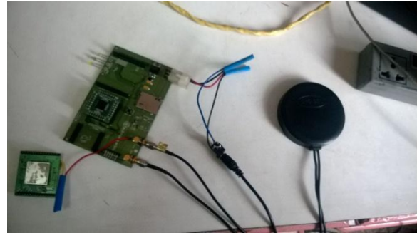
Fig.8. raspberry pi with GSM &GPS
