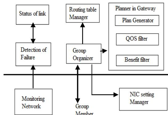
Fig.2. ARS Software Architecture
