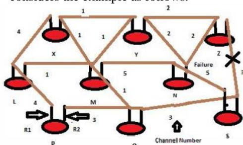
Fig.3. Multiradio WMN undergoes wireless link failure and requires reconfiguring its setting.
