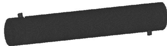
Fig 3.2 Meshed STHX model
