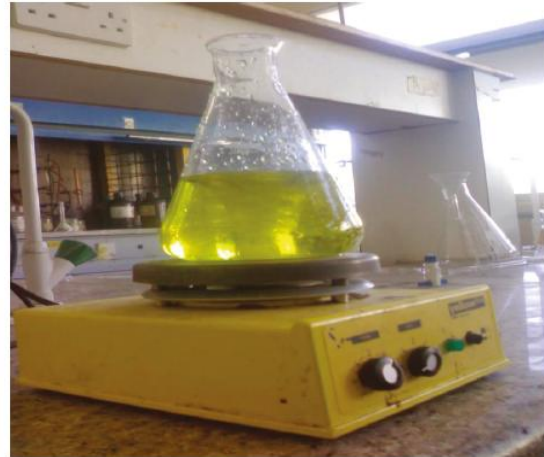
Fig.1. shows solving of catalyst mixture in oil (60°C 1250rpm)
