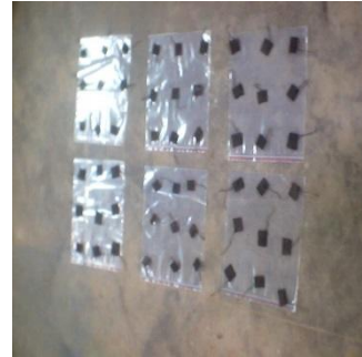
Fig-5 Test coupons from 3 sections of laminate
