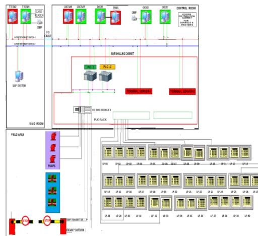
Whole Plant Is Controlled By PLC PANELS and This SYSTEM ARCHTECH. Explains the whole Controlling System.
