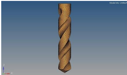
Fig 9.2 104° point angle drill bit
