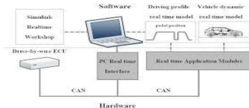
Fig. 2: ECU software test setup using simulation for testing software.
