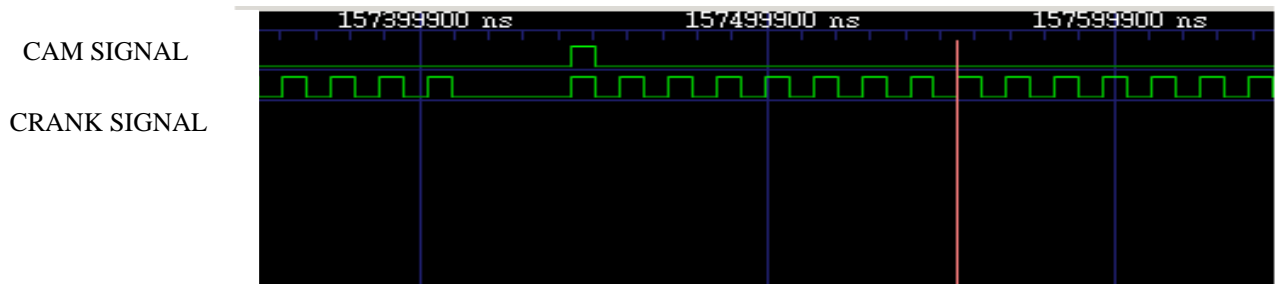
Fig.4: Generated crank and cam signal during Engine Crank.
