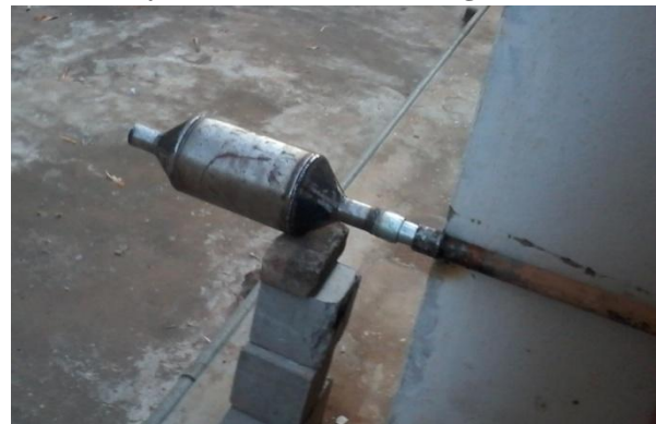
Fig.12: Catalytic convertor fitted to engine
