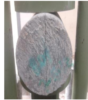
Fig.10.1. Testing of cylinders
