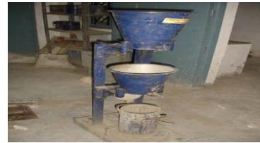
Fig.8.2. compaction factor test
