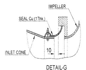
IMPELLER SEAL DETAIL
