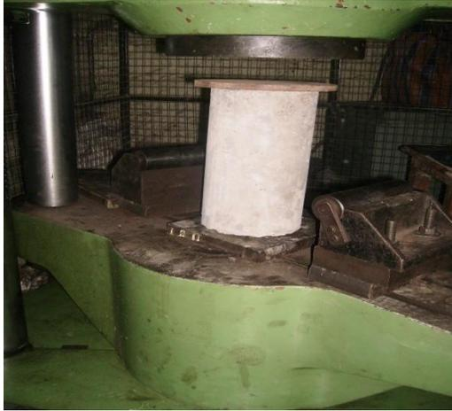
Placing of Mould on U. T. M.
