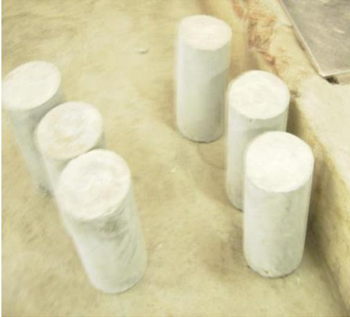
After removing from mould
