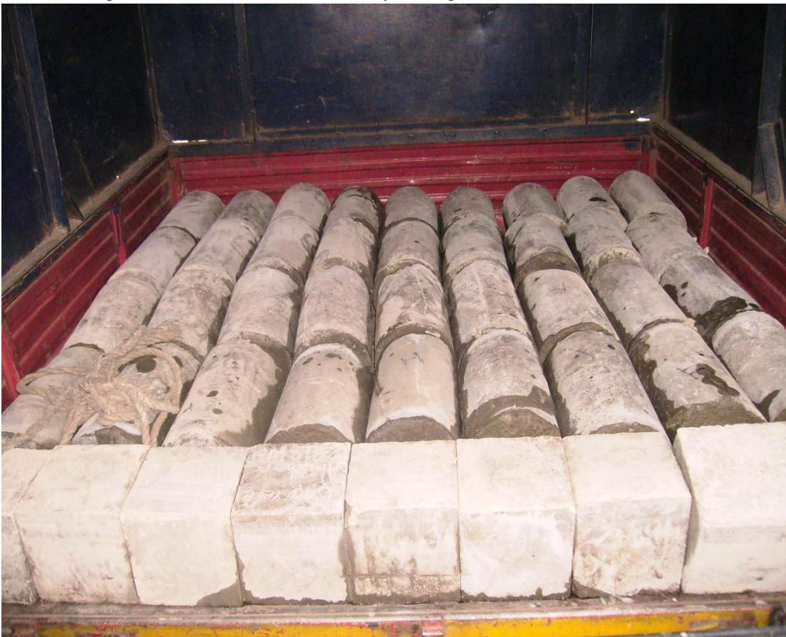
Carrying out 36 moulds to Durocrete Lab Compressive and Split tensile strength testing
