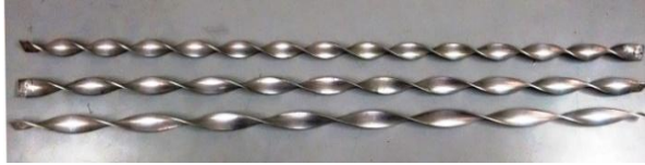
Fig. 2 Twisted Tape Inserts of y=3.0, 4.0, 5.0
