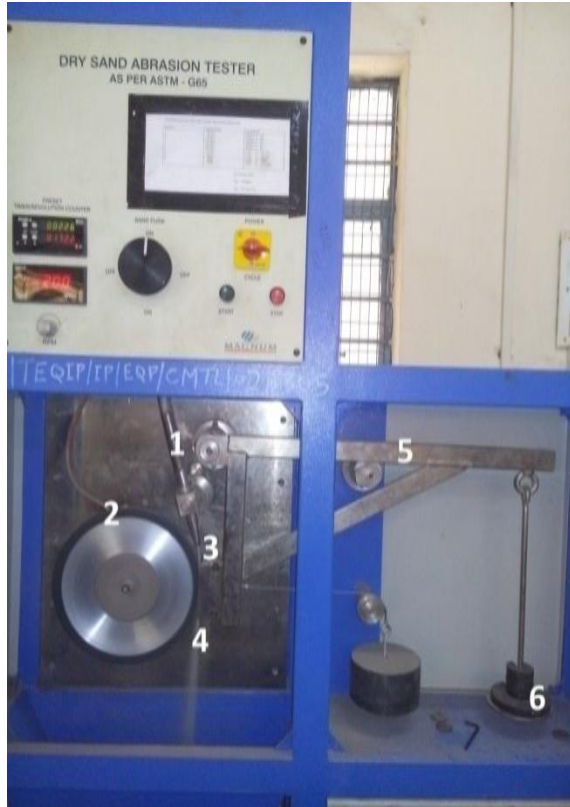
1.Nozzle, 2.Rubber lined wheel, 3.Specimen, 4.Silica sand, 5.Lever arm, 6.Weights
