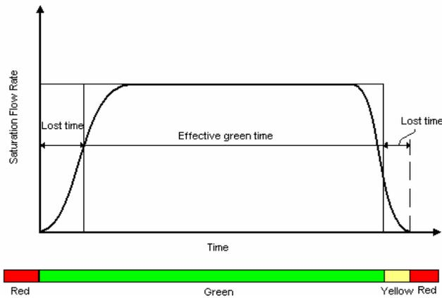
Fig. 1 The flow of traffic during the green period from a saturated approach
