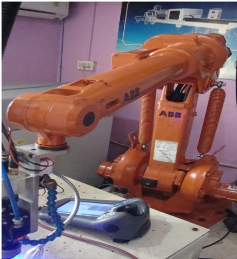
Fig. 1. Experimental setup showing Nd:YAG laser welding machine.
