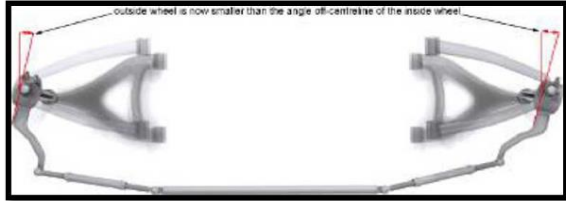
Fig 4.2 - Ackerman steering geometry
