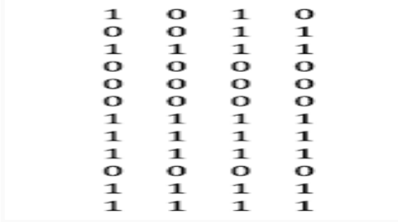
Fig. Example syndrome values for errors that effects first data bit in the proposed bit placement
