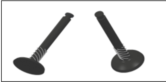
Fig 4: Swirl generated inlet valve
