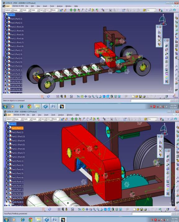
Model arrangement of cutting mechanism in CATIA-V5
