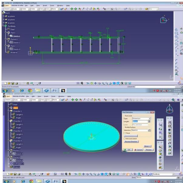
Using Pad Command for thickness
