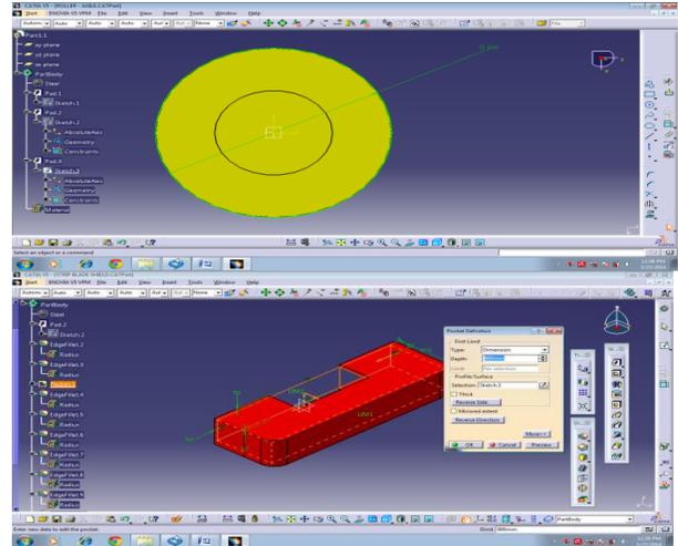
Using Pocket Command for thickness
