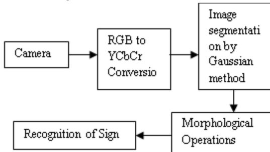
**Fig 1: Block diagram of decoding the sign language.**
