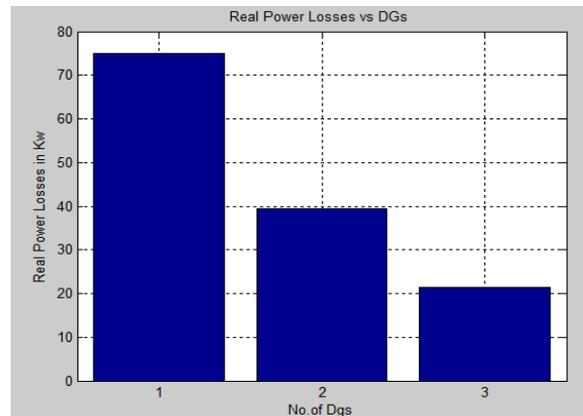
Fig5.7.Real Power reduction using Backtracking Search Algorithm (1DG, 2DG, 3DG)
