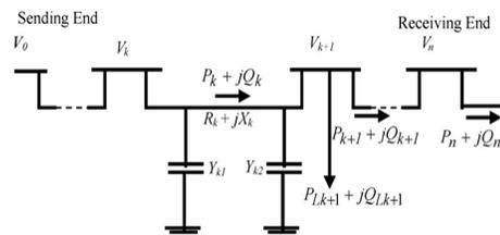
Figure 2.1: Single line diagram of a main feeder
