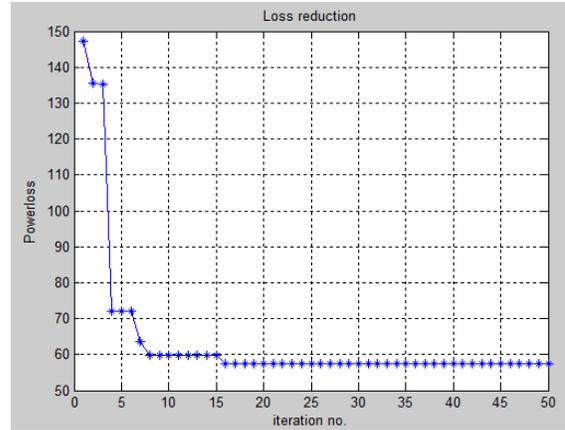
Fig. 5.3. Active power loss versus iteration of 33- bus feeder.
