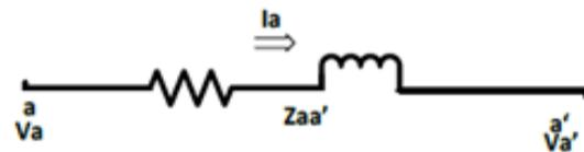
Fig4.1: Typical Single Phase Feeder
