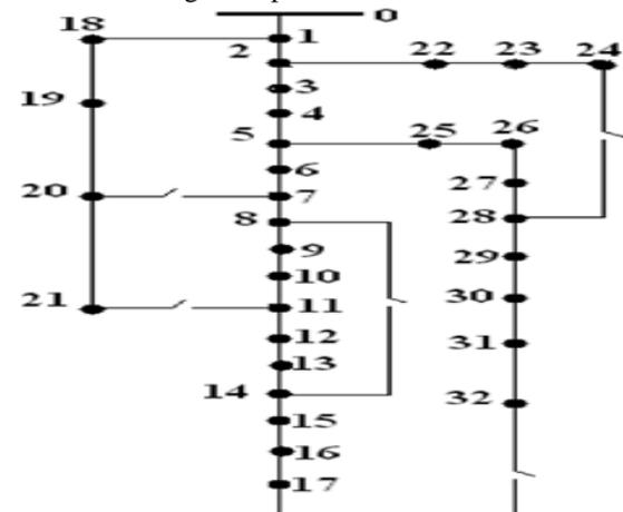
Fig. 5.1 Layout of the 33-bus feeder.
