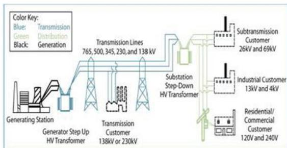
Fig 1.1 Diagram of a distribution system
