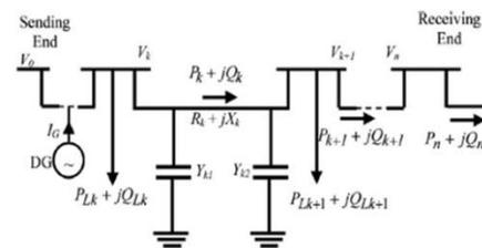
Figure 2.2: Distribution system with DG installation at an arbitrary location
