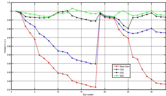
Fig.5.6: Voltage profile before and after DG placement for 33 bus system
