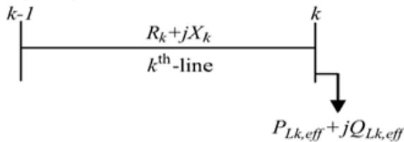
Fig 3.1: connected line between bus k-1 and k
