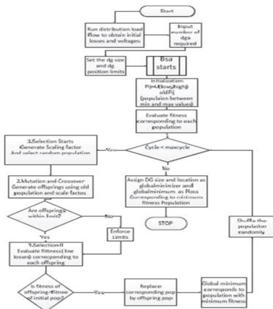
Fig. . Flowchart of BSA for optimal DG placement.
