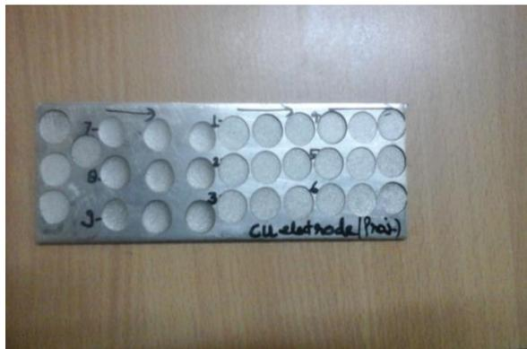
Figure 2: Work piece of Inconel 718 after machining with Cu electrode
