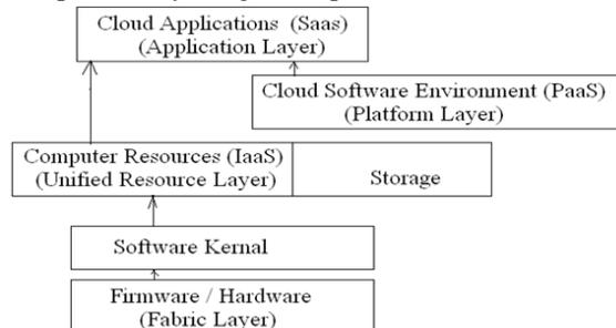
Figure 3:- System Architecture of Cloud Computing
