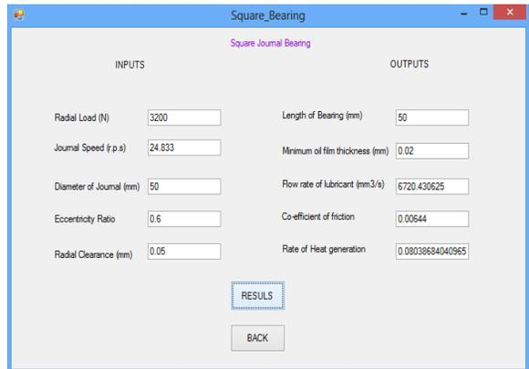
Fig.7 Outputs of Square Bearings
