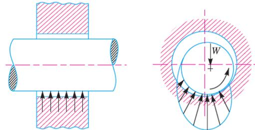
Fig.2 Pressure Distribution in Hydrodynamic Bearing<sup>[2]</sup>
