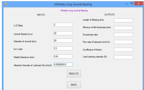
Fig.8 Inputs of Infinitely Long Journal Bearings
