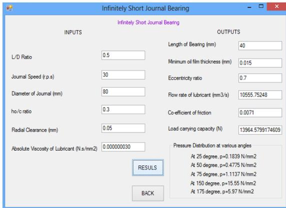
Fig.5 Outputs of Infinitely Short Journal Bearings
