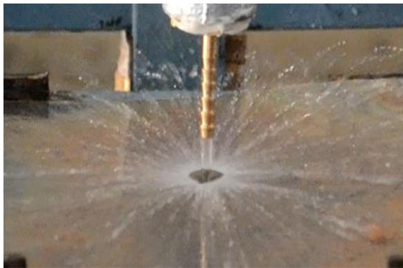
Fig. 3 Image of coolant flow over hot surface
